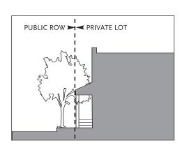
**C. Stoop:** the façade is placed close to the frontage line with the ground story elevated from the sidewalk, securing privacy for the windows. This type is suitable for ground floor residential uses at short setbacks. This type may be interspersed with the shop front. A porch may also cover the stoop.
