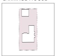
carriage house is an architectural type consisting of a stacked dwelling unit over a garage. It is typically located on an alley at the back 20% of a lot that includes a main house.
