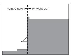
**B. Shop front:** the façade is placed at or close to the right-of-way line, with the entrance at sidewalk grade. This type is conventional for retail frontage. It is commonly equipped with cantilevered shed roof or awning. The absence of a raised ground floor story precludes residential use on the ground floor facing the street, although this use is appropriate behind and above.
